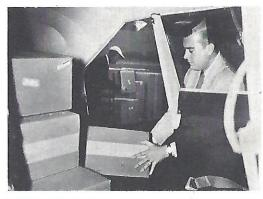
PERFECT FOR CARGO Many business firms and farmers find the Tri-Pacer is ideal for carrying cargo. With the rear seat removable in 15 seconds, there is 42 cubic feet of space available. Large bulky articles can be easily loaded through the separate rear door. Up to 600 pounds capacity.
