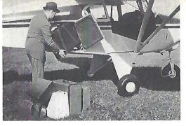
AMPLE BAGGAGE SPACE There's room for all this baggage, 18 cubic feet of it, in the Tri-Pacer. Large separate baggage door makes it easy to load and unload. Hat shelf above baggage compartment is easily removable to provide additional stowage space if needed.
